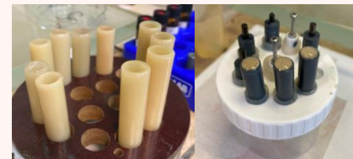
Membrane formation: on the left – it is fixed with glue, on the right – formed by drop-casting
